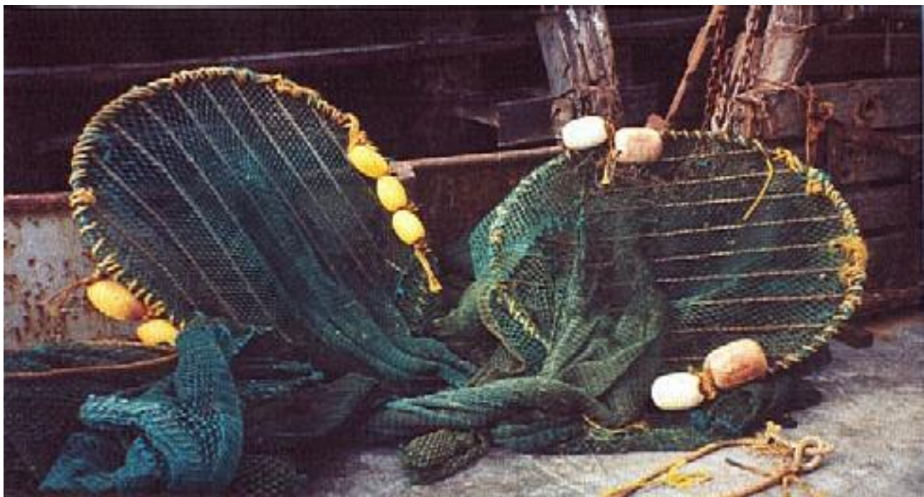
Photo 1: Super shooter TEDs on a Sea Bob trawler (Paramaribo, Suriname), by Luc Laurent
